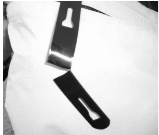
Figure 9-4. Broken Strap After First Use
