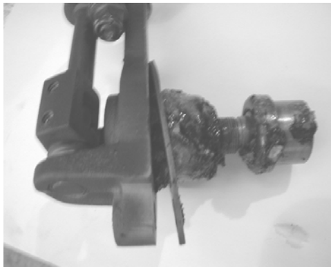
Figure 8-8. Sludge on shutter control
